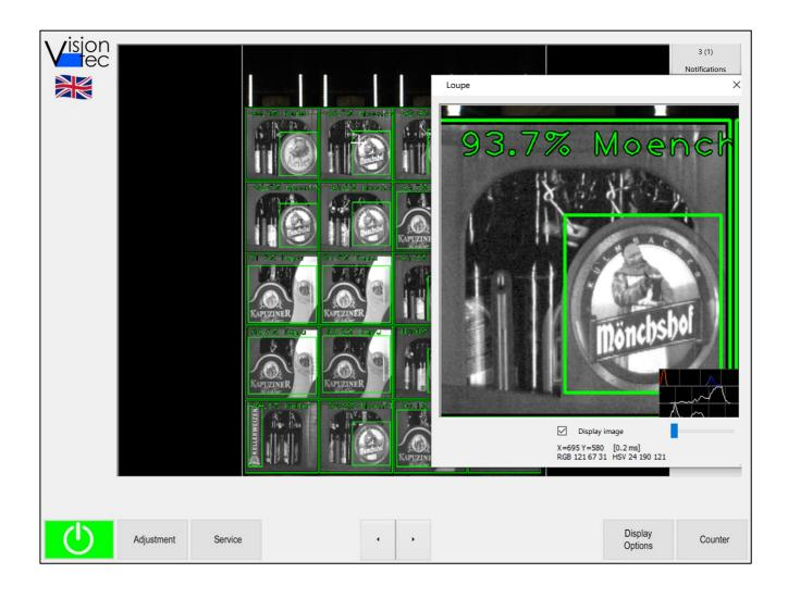
With the side camera systems, side stacks of crates on the pallet are inspected - in the case of the Euro pallet, this means all crates.
